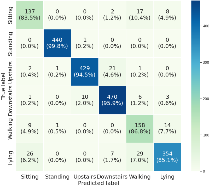
FIGURE 5.9. Confusion matrix for the estimation of 6 activities using LSTM.
