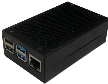
FIGURE 3.19. Gateway/aggregator node expressed by a Raspberry Pi 4 B
