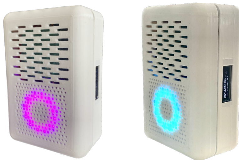
FIGURE 3.15. 2 nd Prototype of the air quality assessment node, and 2 feedback states: a) Calibration phase; b) Good air quality levels.
