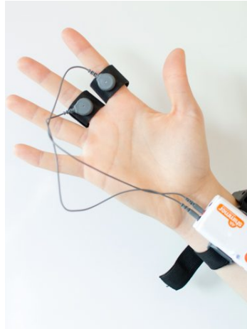
FIGURE 3.12. Shimmer3 GSR+ unit and the electrodes placement on the hand. Source: [205]
